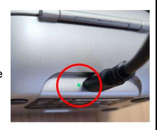
When the hearing aids are charging a light will flash, this might be red, amber or green – any flashing colour means the aid is charging
