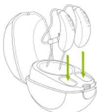
The indicator light will show the charging state of the battery until the hearing aid is fully charged. When fully charged the indicator light will remain on, i.e. solid green light.
