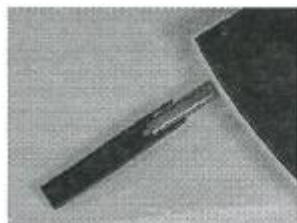
Picture 1: strip holder and metal sled (bottom view)
