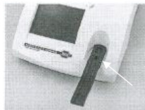
Picture 3: check alignment of sensor windows
