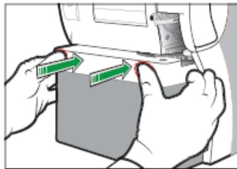
Figure 4 – inserting new solution pack
