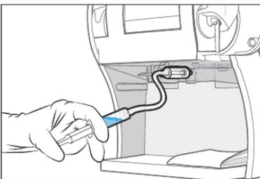
16. Inject a very small quantity of air to fill approximately 1 cm of the tube.
