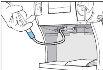
18. Inject a very small quantity of water to fill approximately 1 cm of the tube.
