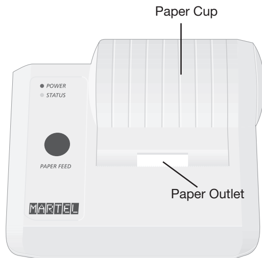
Top view of Martel Printer
