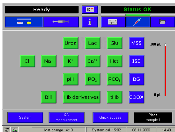
Figure 6-10 Analyzer mode screen when Aspirate from syringe mode is activated
