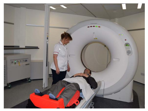
The patient is positioned on the CT scanner and accessory equipment is used such as a footstock, angled boards or individually made head shells to ensure that the patient will be able to remain still and in a reproducible position for the duration of their treatment course
