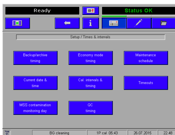
Figure 10-A Times & intervals screen in Setup mode
