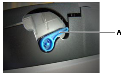
A Printer lever "down" position
