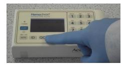
Press the 'QC' button and select the correct level as displayed on-screen:
